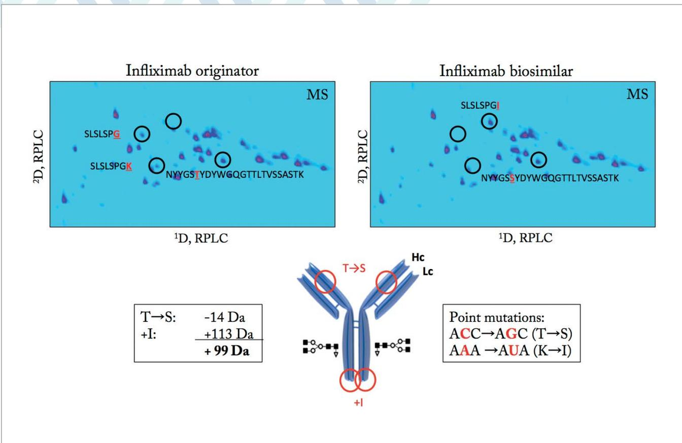
The power of advanced analytical tools. RPLC×RPLC-QTOF-MS analysis of infliximab originator and candidate biosimilar. Drawing of the mAb with annotation of the modifications. Courtesy of the Research Institute of Chromatography ([www.richrom.com](http://www.richrom.com)).
