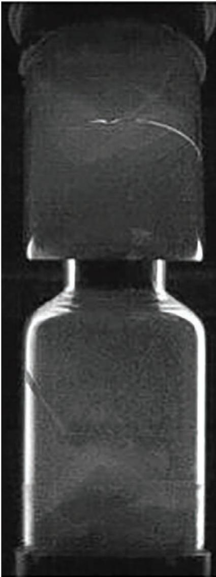
Figure 2: The glass wall of the vial acting as a light guide
