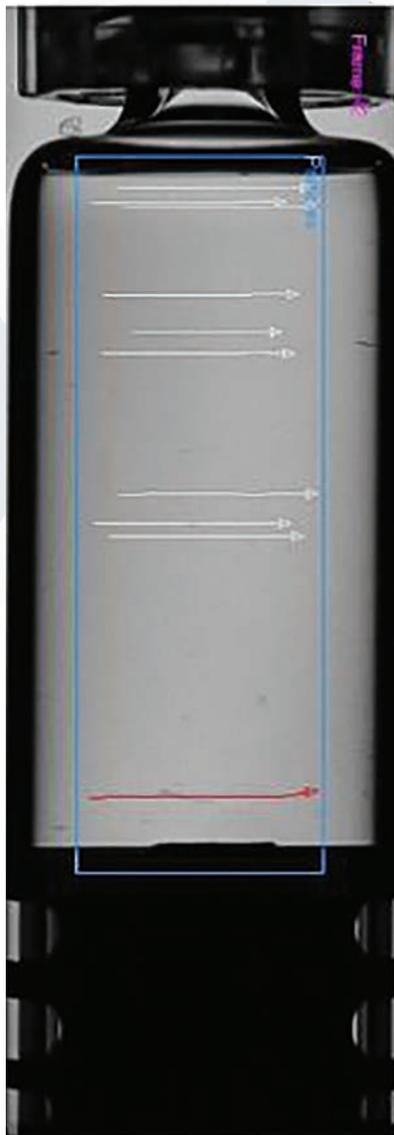
Figure 3: The apparent rotation speed of the potential contaminants is used to determine if they are inside or outside of the liquid
